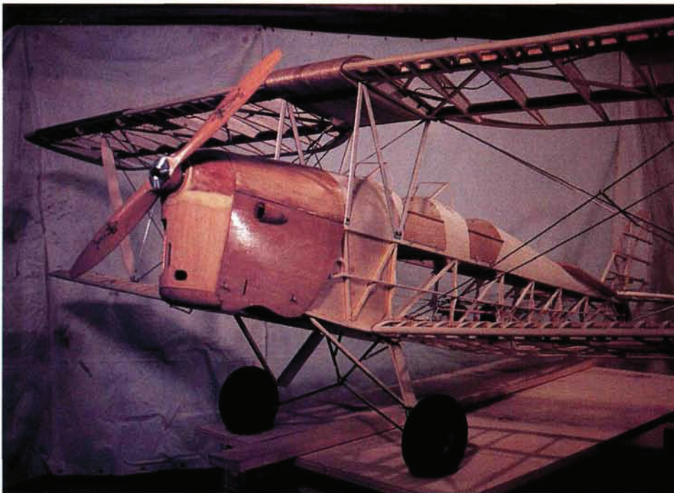
Top: the Tiger Moth model construction closely follows the method used to build the full-size aircraft. It includes traditional use of balsa, plywood and lite-ply. Center: the engine cowl and the cabane struts and top wing center-section structure. Bottom: nothing complicated here. The tail surfaces are light and strong. Notice the filler blocks used around the Robert HingePoint hinges.
