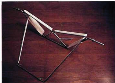
The functional landing gear is scale but not difficult to build. It is made of bent and soldered music wire, and rubber bands are used for shock absorbing.
