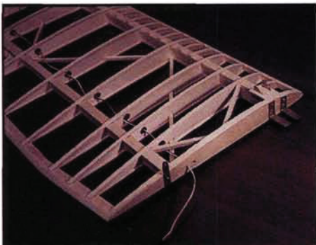
The wing structure is relatively simple and uses a scale flat-bottom airfoil. Notice the internal diagonal bracing.
