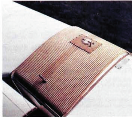
The top wing center section on the full-size aircraft was also the main fuel tank. The author used long strips of balsa, plywood, small pieces of brass and aluminum tubes and some miniature screws to replicate the finest details.
